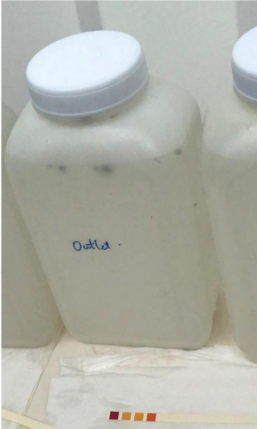
Water sample was collected at the stormwater terminal discharge point on 20 December 2018, and the pH tested with pH paper was approximate 1-2.
